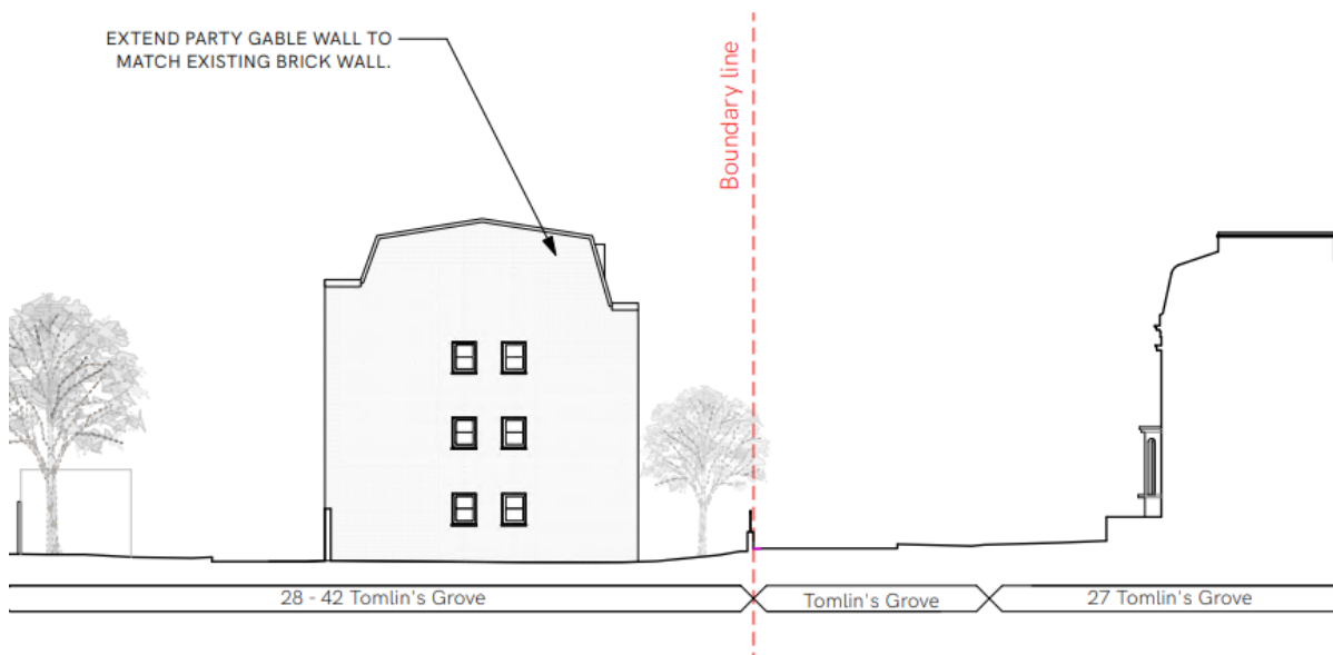
Figure 3: Proposed north elevation showing the relationship with the adjacent terrace on Tomlins Grove
